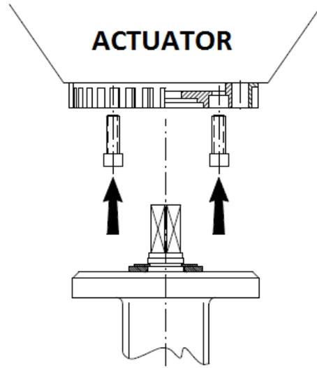
Screw the flange to the actuator with hexagon socket screws
