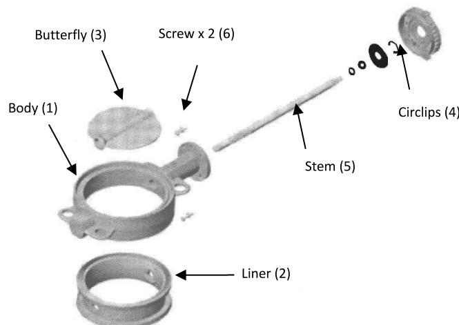
Remove the motor actuator. Unscrew the screws (6), remove the circlips (4). This frees the shaft (5), thus enabling the liner (2) and the butterfly (3) to be taken out of the body (1). Replace the worn parts: To obtain the list of spare parts for every valve, please contact our technical department at: +33 (0)474 94 90 70
