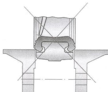
The liner can get damaged if the counter-flanges are not sufficiently spaced.
