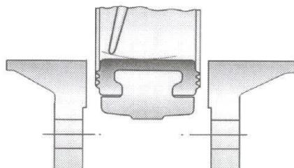
The gap in-between flanges has to be large enough to allow the valve be inserted without the elastic liner getting caught. The butterfly has to be in an almost closed position.
