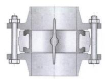
The butterfly has to be in the fully open position after positioning the valve in-between the counter-flanges and before tightening the bolts, otherwise the elastic liner might be deformed or deteriorated during the tightening of the first manoeuvre.
