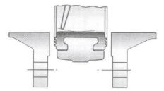
The gap in-between flanges has to be large enough to allow the valve be inserted without the elastic liner getting caught. The butterfly has to be in an almost closed position.
