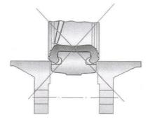
The liner can get damaged if the counter-flanges are not sufficiently spaced.
