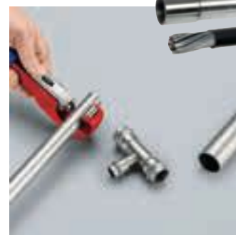
For cutting copper, brass and stainless steel pipes and rigid steel conduits with wall thickness up to 2 mm
