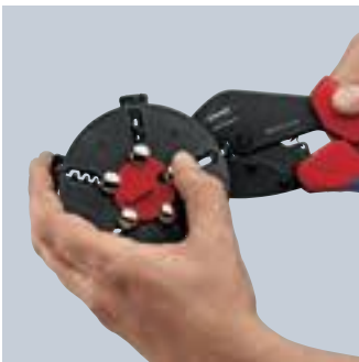
Changing the crimping dies: unlock the magazine position, take out the set of dies which the pliers have been pushed on
