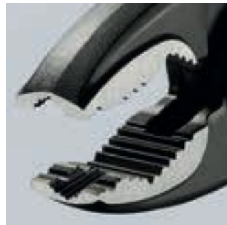
Optimised jaw geometry: 2-zone gripping jaw with opposing alignment of teeth – for maximum grip when loosening and tightening.
