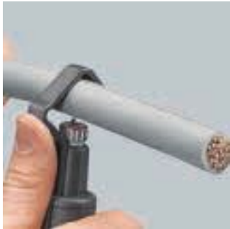
Setting the tool for circular cut
