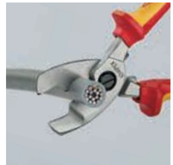
Final cut: after cutting the sheath in the front profile the conductors in the rear part are cut. Initial cut in the front profile, final cut in the rear profile – to keep it as easy as possible.
