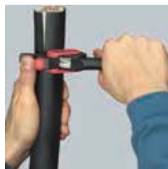
Turning the tool for circumferential cut
