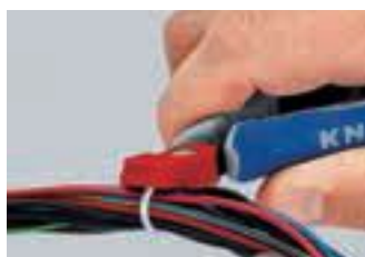
Remove the head of the cable tie using the Electronics Diagonal Cutter...
