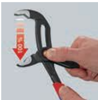
Press the button – open pliers completely
