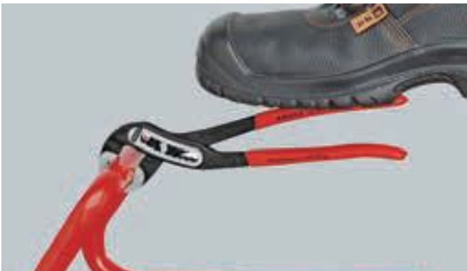
Self-locking on pipes and nuts: no slipping on the workpiece; the complete actuating force can be used to turn the workpieces; not having to squeeze the pliers handles reduces the required effort
