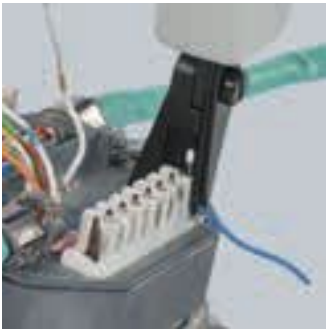
Inserts and cuts cables in one operation
