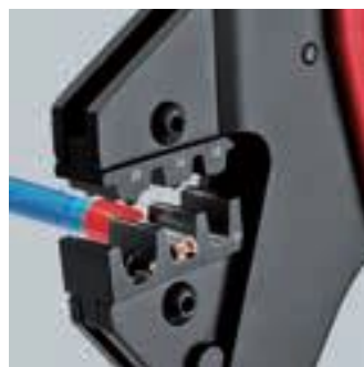
97 43 200 with crimping dies 97 49 09 for wire ferrules
