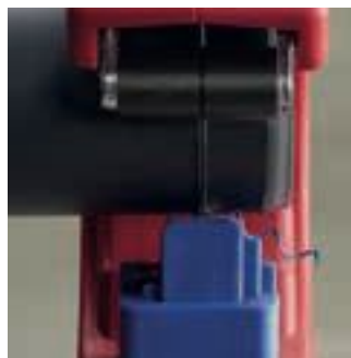
Segments as short as 10 mm can be cut. The spiral chip comes from chamfering
