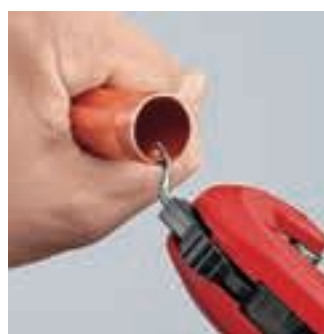
And you're done! If necessary, have the edge smoothed out using the fold-out deburring tool – with surprisingly little effort
