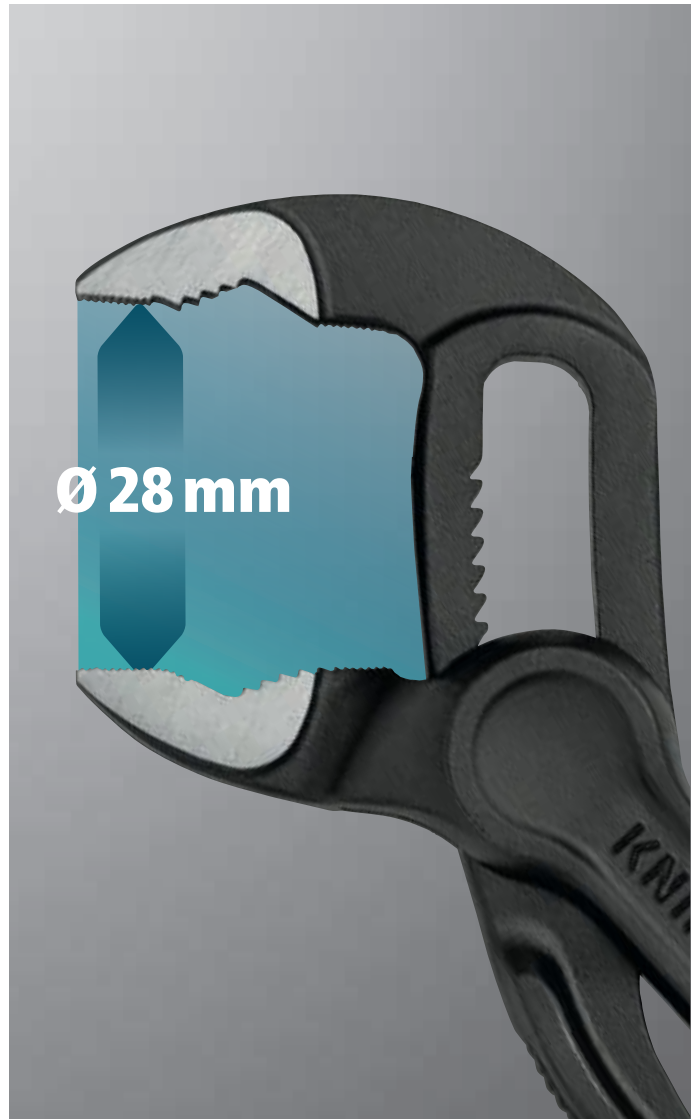
Naked truth: The grips are not coated to keep them as slim as possible. To ensure good grip, they are textured on the outside
