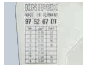
Position settings for the crimp depth can be clearly read on the pliers
