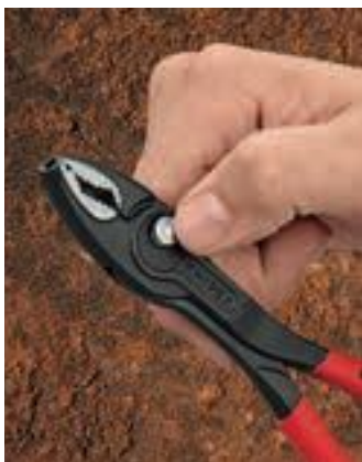
The KNIPEX TwinGrip allows the gripping capacity to be set flexibly in five positions...
