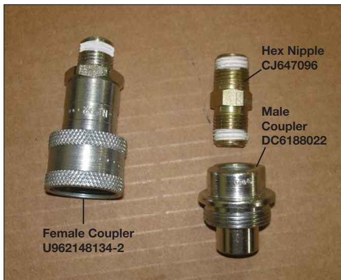
Figure 5, New 1/4 NPTF Couplers (10,000 PSI/700 Bar Models)
